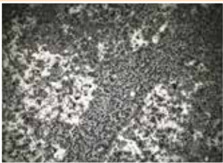
Magnitude picture of A1 panels with A1 Sealer after 4 years on sunny side.
