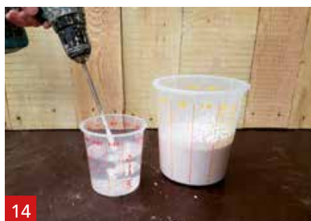
11 Gently add the A1 Powder to the A1 Liquid.
