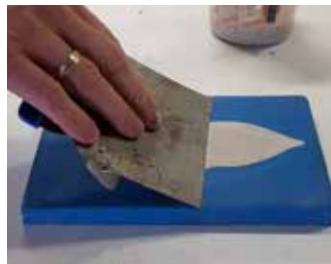
Pour the desired amount of A1 into the mould and scrape away the excess A1 with a putty knife.
