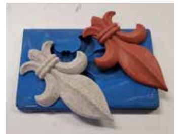
Result after drying and unloading; a solid cast object, an exact copy of the mould.
